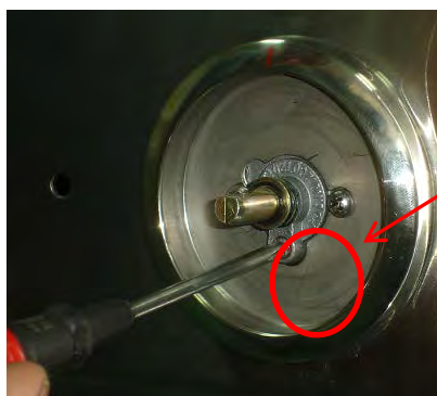
Low flame setting screw (where applicable)
