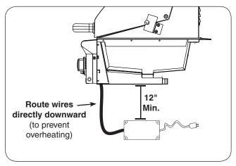
Fig. 15-3 Power supply clearance
