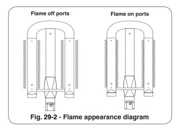
the air shutter until the flames appear to burn while touching the burner ports (Fig. 29-2). If flames are a lazy yellow, open the air shutters until the flame is mostly blue.
