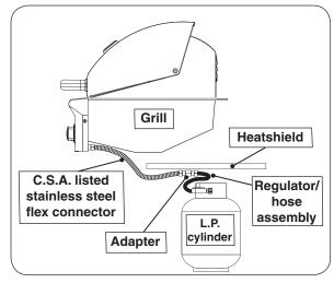
Fig. 12-2 Propane cylinder orientation
