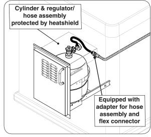
Fig. 12-3 Optional AOG door w/tank tray
