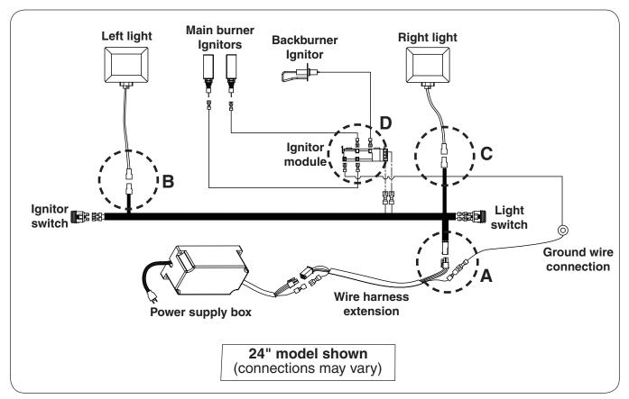
Fig. 32-1 - Wire diagram
