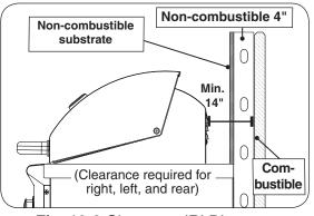
Fig. 10-3 Clearance 'B' Diagram
