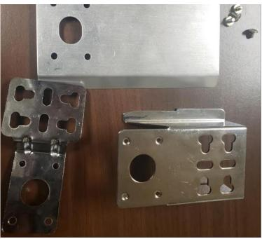
2. Line up the large opening and corresponding screw holes of the Motor Mount, Bracket, Housing Cover. Secure with the 4 Housing Cover Screws (as shown below).
