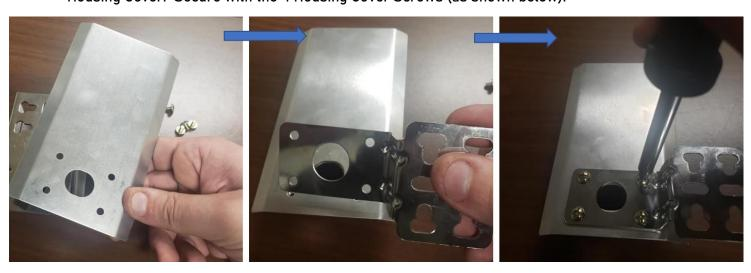
3. Bring your Mount Assembly close to your stand and line up the lower part of the bracket to your desired height facing the outside of the stand. The large opening should line up with the notch in the stand. Secure the assembly in place with 2 bracket screws/nuts (as shown below).
