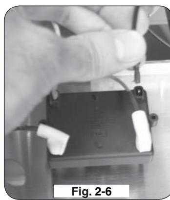
Connect wire to the ignitor module
