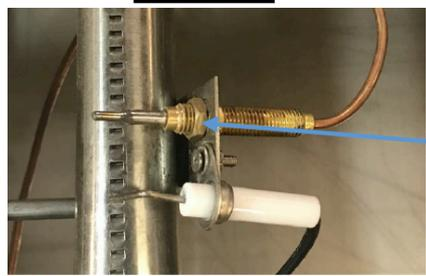
Remove Nut From Thermocouple Then Pull the Thermocouple Out From The Bracket. Note the Position of The Tip of The Thermocouple Before Doing So.
