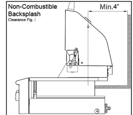
**Clearance between grill and protected combustible wall** (i.e. a non-combustible wall in front of a combustible wall to serve as a barrier. This can be accomplished by brick or a metal stud finished with non-combustible substrate. Clearance Fig. 2). The grill must have a minimum of 14" right, left and rear clearance from the protected combustible wall. (The 4" non-combustible material clearance, plus an additional 10" clearance between the grill and protected wall.)
